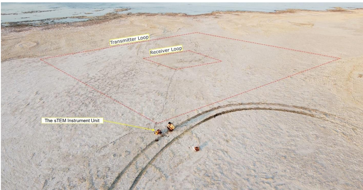
Figure 4 Configuration of the sTEM system.
