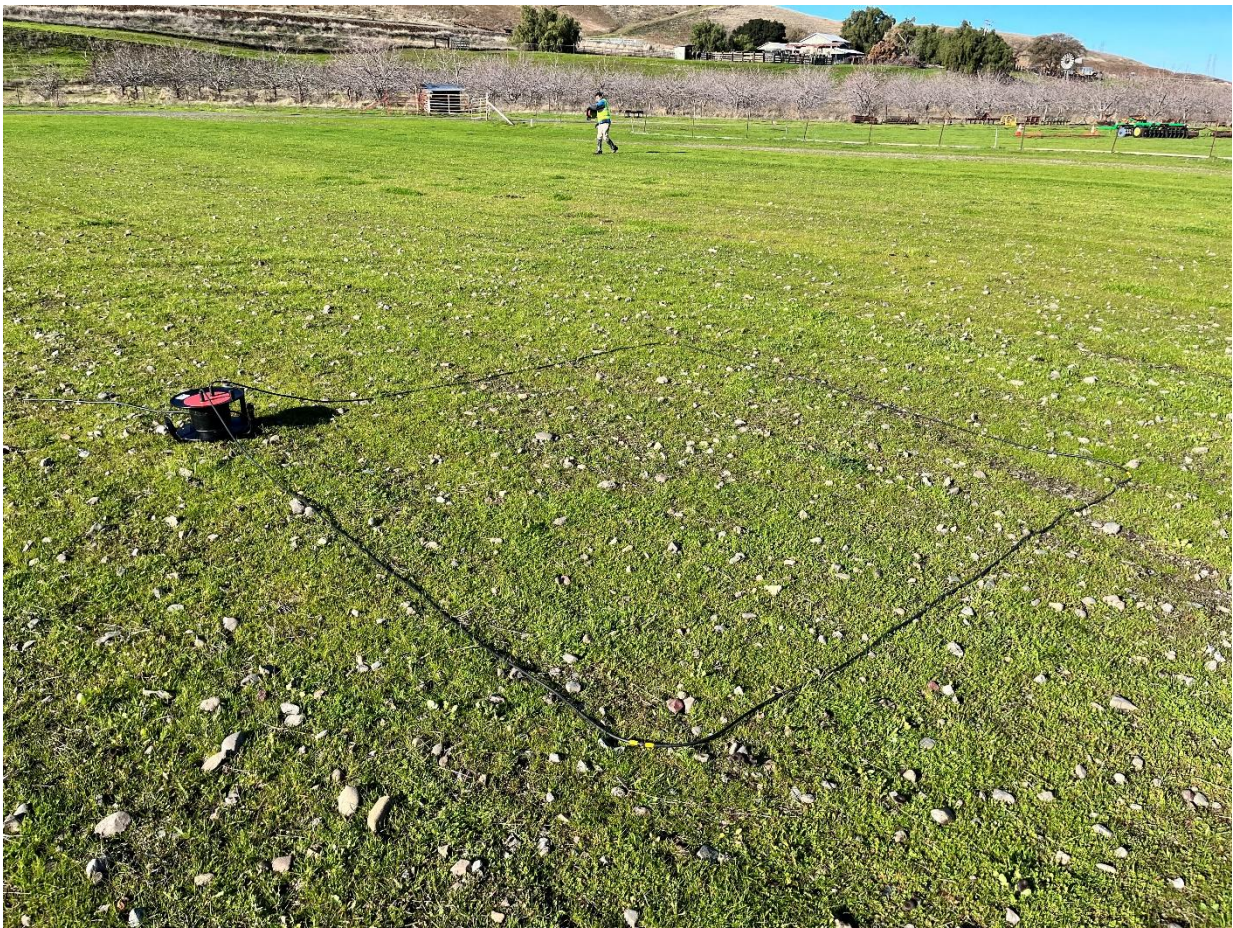
Figure A2- 5 The 3x3 m receiver loop installed in the center.
