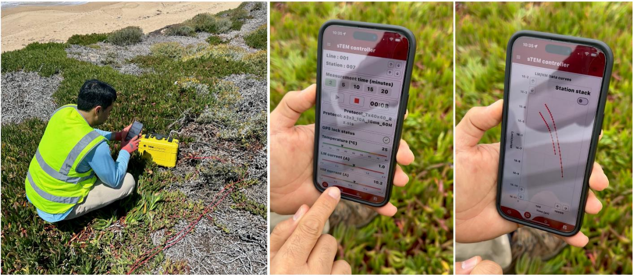
Figure 6 Photos from the field. (left) The sTEM system in operation. (right) data acquisition controlled in real time from a cellphone.
