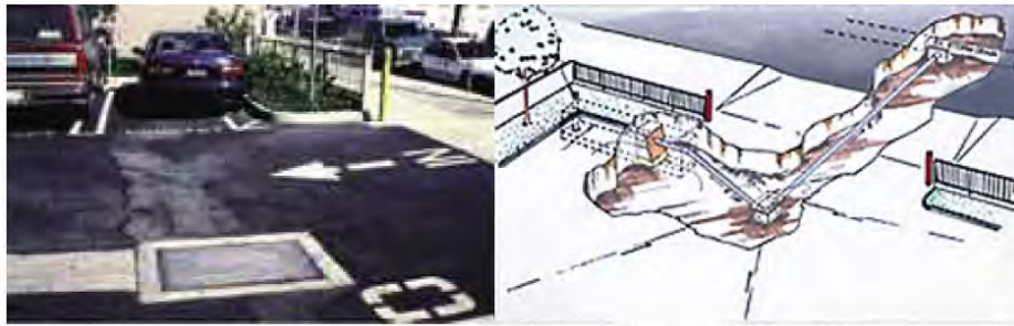
Picture and schematic drawing of parking lot infiltration (Source: Louisiana Department of Transportation)
