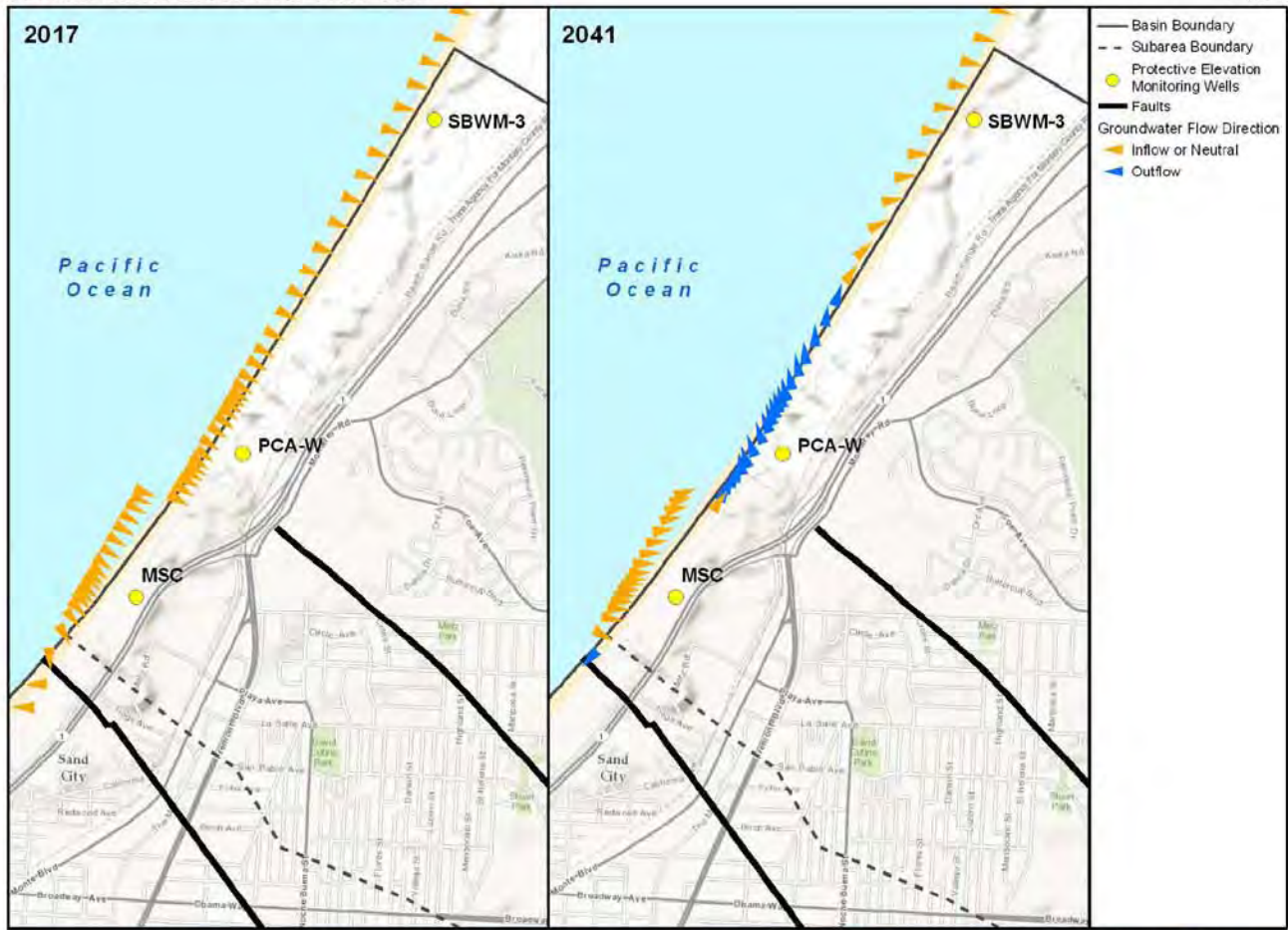
Figure 7: Layer 4 Average Flow in 2017 and 2041 for Scenario2 to Achieve Protective Elevations within 25 Years
