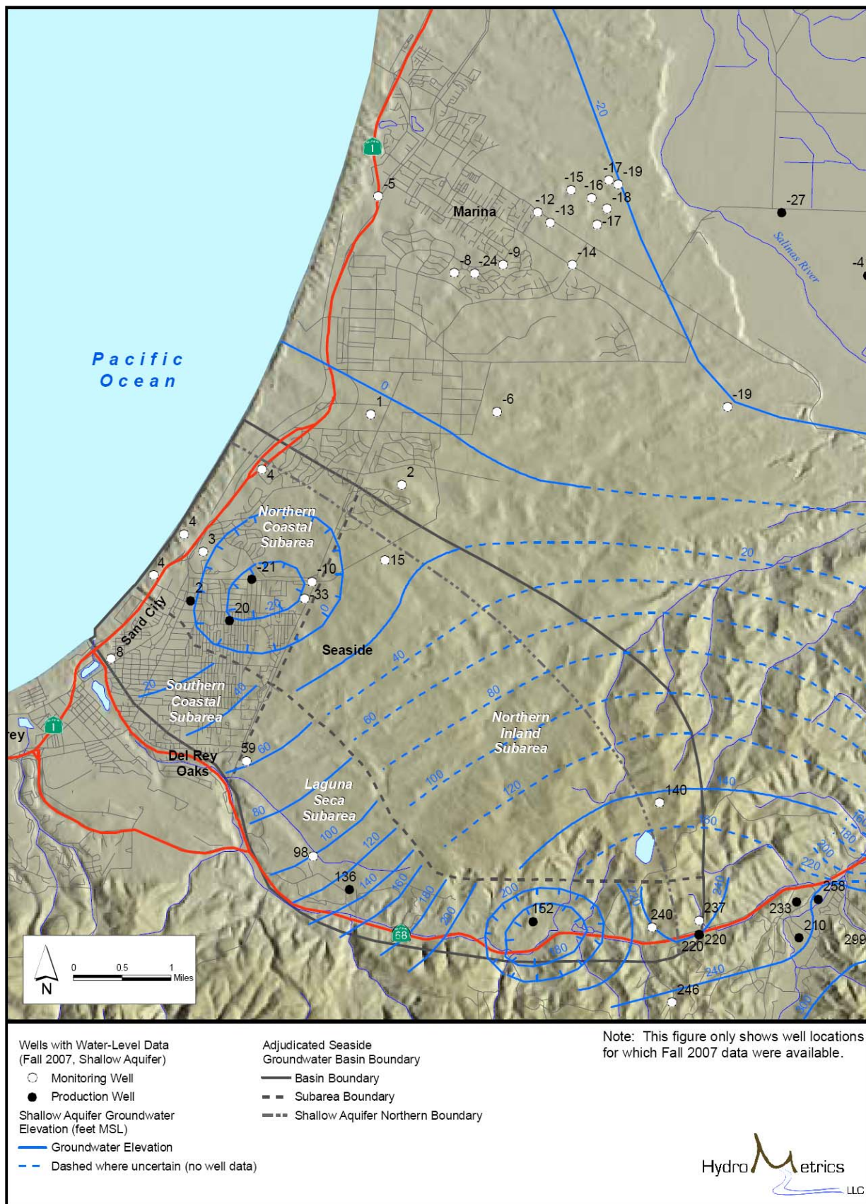
Figure 5: Groundwater Elevation Contours in the Shallow Aquifer (Correlated to the 400-Foot Aquifer in Salinas Valley) – Fall 2007
