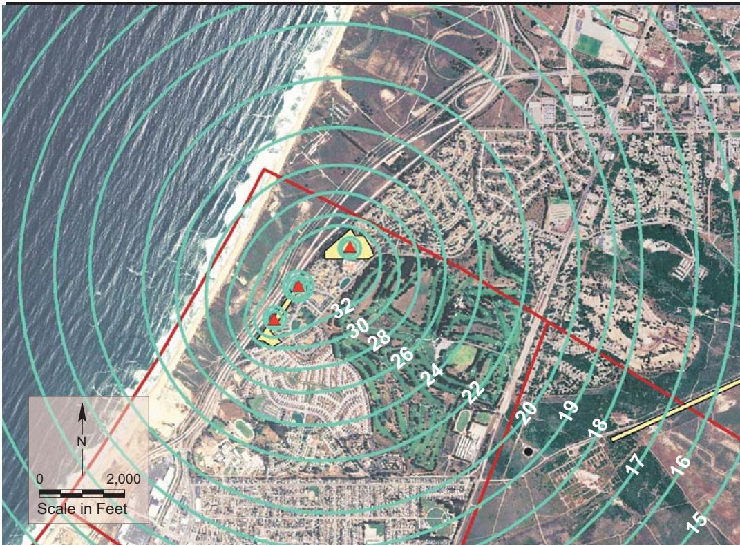
Injection Wells - Santa Margarita Aquifer Predicted rise in water levels (ft) after 5 months of recharge at 1,000 gpm/well
