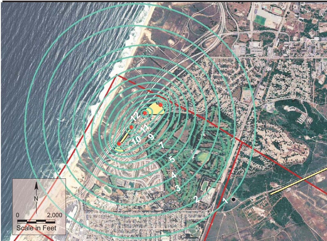
Vadose Zone Wells - Aromas/Paso Robles Aquifer Predicted rise in water levels (ft) after 5 months of recharge at 150 gpm/well
