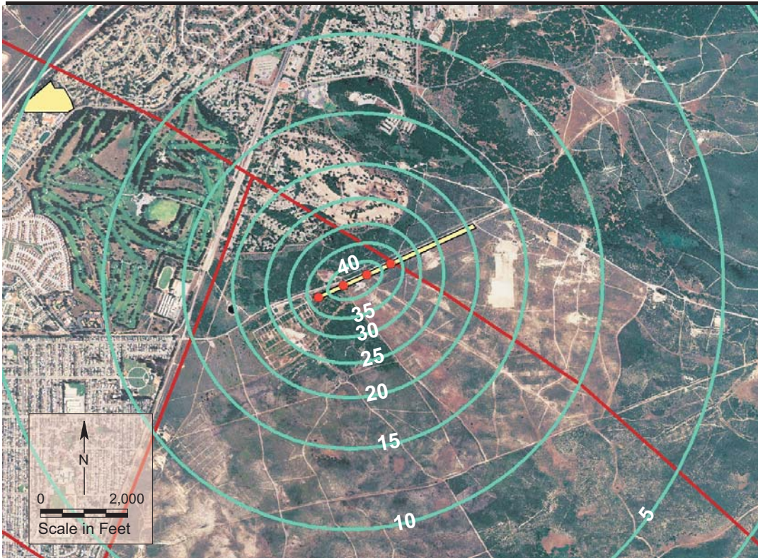
Vadose Zone Wells - Aromas/Paso Robles Aquifer Predicted rise in water levels (ft) after 5 months of recharge at 400 gpm/well
