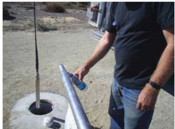
Down-hole Water Sample Collection
